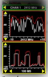
Measure frequency response over time to identify roque wireless energy sources
