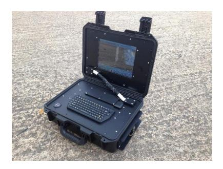
The moulded ABS case version has on-board batteries and an integrated screen and keyboard and can be used in all weathers, in the open position.
